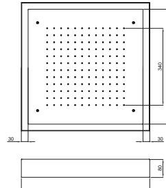
*Ceiling-mounted 304L stainless steel shower head, 570 mm square with anti-limescale nozzles, equipped with a rain shower jet and LED lighted chromotherapy and G1/2" connection.*
