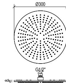
*Round shower head, 30 cm diameter in 316L stainless steel, inspectable, with anti-limescale nozzles and G1/2" ball joint connection.*
