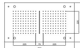
*Recessed 304L stainless steel shower head, rectangular 700x400 mm with anti-limescale nozzles, equipped with a rain shower jet, cascade jet and LED lighted chromotherapy, G1/2" connection, fastening with frame and safety stays.*
