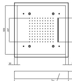
*Ceiling-mounted 304L stainless steel shower head, 570 mm square with anti-limescale nozzles, equipped with rain shower jet, mist shower, waterfall shower and LED lighted chromotherapy, G1/2" connection.*
