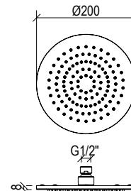
*Round shower head, 20 cm diameter, in 316L stainless steel, inspectable, with anti-limescale nozzles and G1/2" ball joint connection.*
